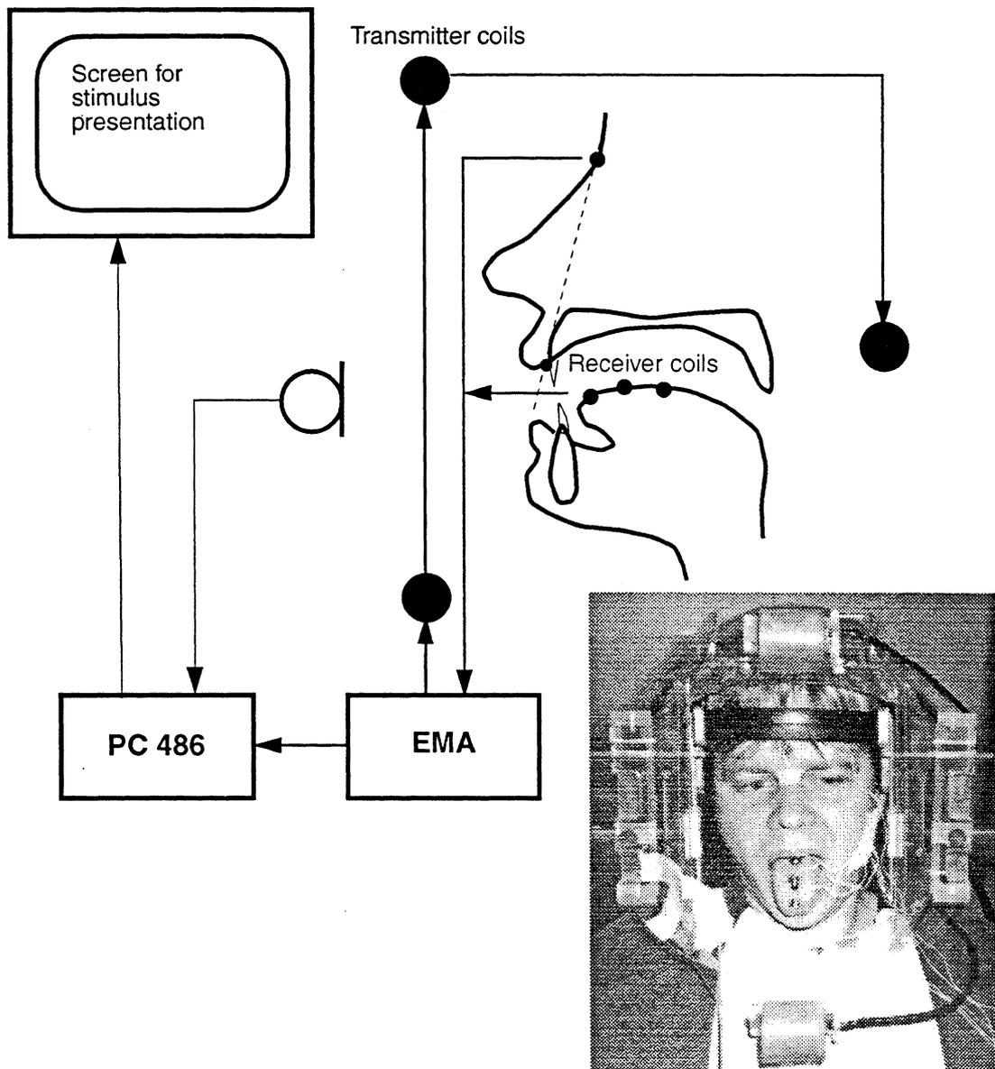
Fig. 5: Experimental setup and placement of receiver coils (bottom right: front view of the subject with tongue stretched out to demonstrate the placement of the receiver coils).
